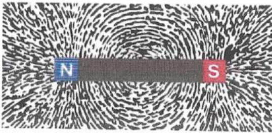
A pictorial representation of the magnetic field which describes how a magnetic force is distributed within and around a magnetic material
